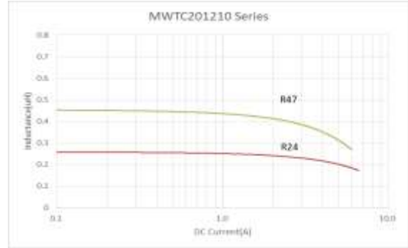
Inductance vs. DC Current Characteristics
