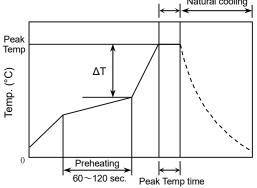
5-3. Recommended soldering peak temp and peak temp duration for Reflow soldering Pb free solder is recommended, but if Sn-37Pb must be used, refer to below.
