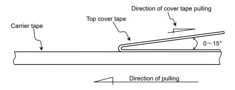
Paper tape should not adhere to top cover tape when pull the cover tape.
