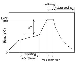
5-3. Recommended soldering peak temp and peak temp duration
