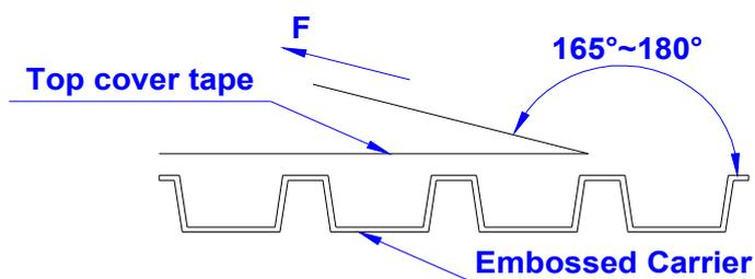
The force for tearing off cover tape is 10 to 130 grams in the arrow direction under the following conditions ( referenced ANSI / EIA - 481 - D - 2008 of 4.11 standard ).
